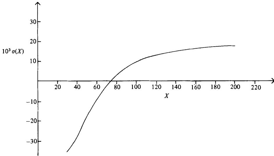
FIGURE 2. The growth-rate function  $\sigma(X)$  corresponding to the initial conditions (3.1) and  $a = 0.069$ ,  $G = 0.025$  and  $\bar{X} = 20$ .
