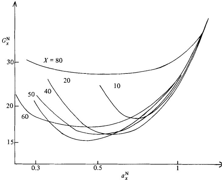
FIGURE 6. The neutral curves corresponding to different locations of the initial conditions (3.1), with  $G = 0.025$ .
