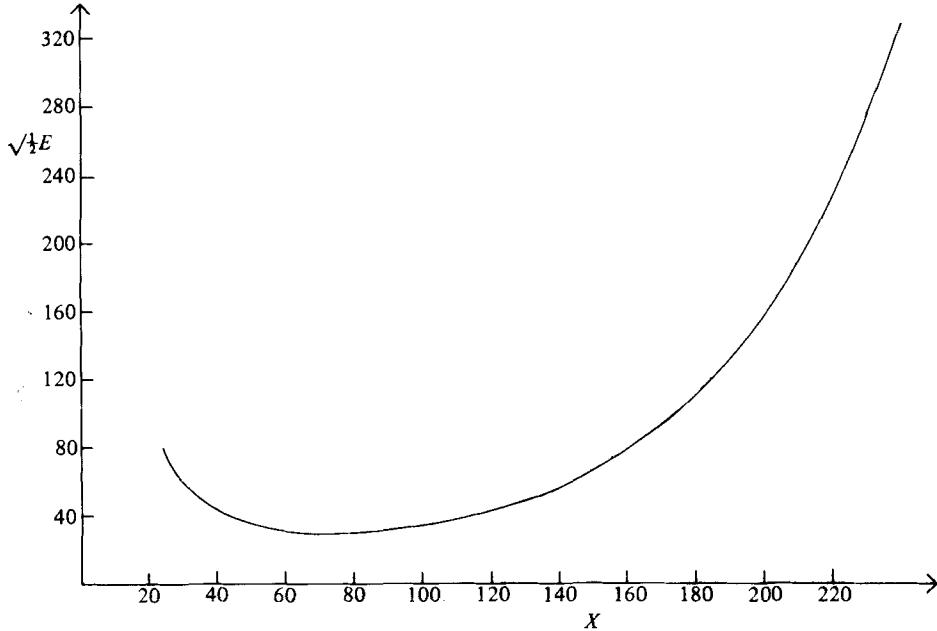
FIGURE 1. The development of  $E$  with increasing  $X$ , corresponding to the initial conditions (3.1) and  $a = 0.069$ ,  $G = 0.025$  and  $X = 20$ .
